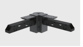
L-shaped Adjustable (Downward) Model: L90-MH20(A) Material: AL6063-T5 Size: L120×W27.2×H52mm (4.72""1.07""2.05") Applicable model: TLS-MH2X0
