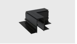
L-shaped (Downward) Model: L90-MR20(C) Material: AL6063-T5 Size: L95×W95×H46.5mm (3.74""3.74""1.83") Applicable model: TLS-MR2X0(C)
