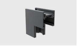
L-shaped (Inward) Model: L90N-MS20 Material: AL6063-T5 Size: L50×W50×H27.3mm (1.97""1.97""1.07") Applicable model: TLS-MS2X0
