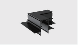
L-shaped (Downward) Model: L90-MR20(B) Material: AL6063-T5 Size: L95×W95×H46.5mm (3.74""3.74""1.83") Applicable model: TLS-MR2X0(B)
