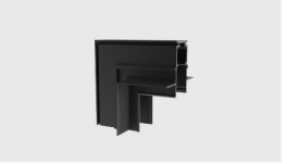
L-shaped (Inward) Model: L90N-MR20(A) Material: AL6063-T5 Size: L80×W80×H64mm (3.15""3.15""2.52") Applicable model: TLS-MR2X0(A)
